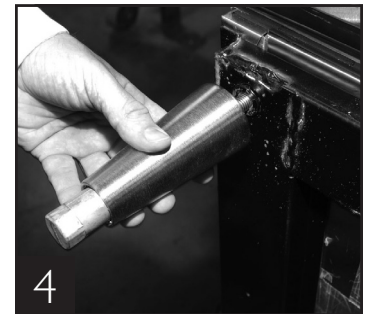
4 Thread leg into cabinet bottom frame rail.
